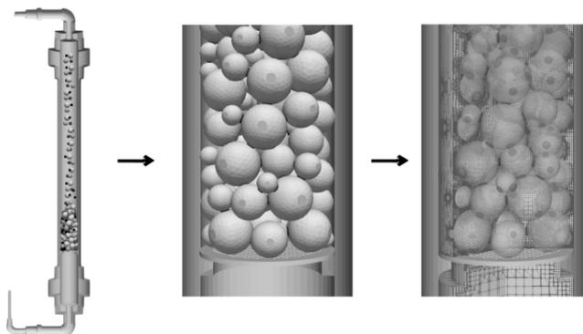
**Fig. 1:** Geometry creation process for a lab scale packing: DEM packing of the particles, scripted adding of the bridges, automated meshing of the volume regions.
